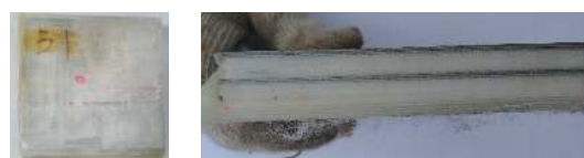
(c) Titanium alloy/UHMWPE composite target
