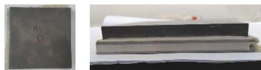
(b) B 4 C/titanium alloy/UHMWPE composite target
