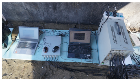
(a) Signal converters and data processing terminals
