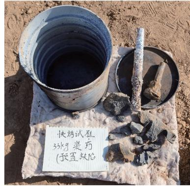
(b) Fragment debris of the Type II cook-off bomb (defect)
