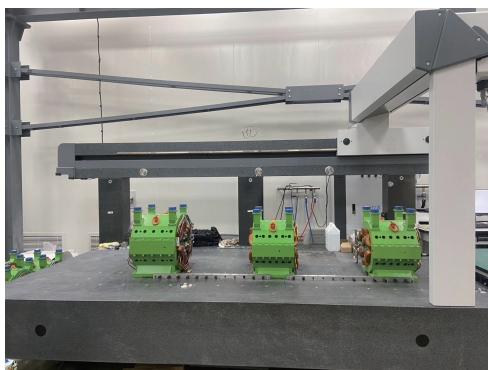
Fig. 1 CMM calibration of magnets
