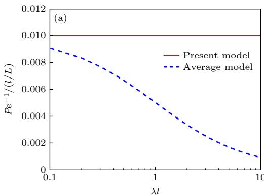
图 5 本模型和 R-平均模型 (average model) 的  $1/Pe^*$  比较 (a)  $C_v = 0.1 (\alpha = 1)$  ; (b)  $C_v = 1.19 (\alpha = 0.8)$ Fig. 5. Comparison of the parameter  $1/Pe^*$  between the present model and the average model: (a)  $C_v = 0.1 (\alpha = 1)$ ; (b)  $C_v = 1.19 (\alpha = 0.8)$ .
