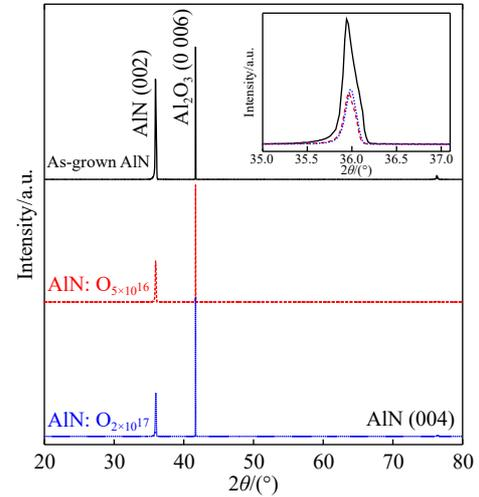
Fig. 1 XRD patterns of as-grown AlN, AlN:O<sub>5 $\times$ 10<sup>16</sup></sub>, and AlN:O<sub>2 $\times$ 10<sup>17</sup></sub>. The inset shows the magnification of AlN (002) peaks.
