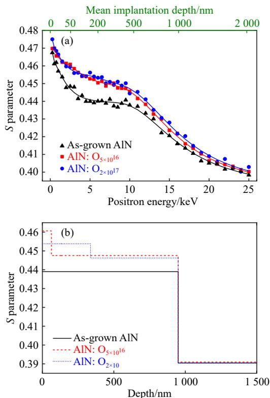
Fig. 3 (a) The parameter S as a function of positron energy (E) for the samples. Solid lines are fitted to the experimental data by VEPFIT software. (b) S depth distributions obtained from analysis of S–E curves for the samples.
