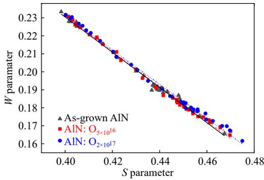
Fig. 4 Plots of  $S$  vs  $W$  for the samples. The black solid, red dashed, and blue dotted lines are fits to the  $S$ - $W$  data for the as-grown AlN, AlN:O<sub>5×10<sup>16</sup></sub>, and AlN:O<sub>2×10<sup>17</sup></sub>, respectively. (color online)
