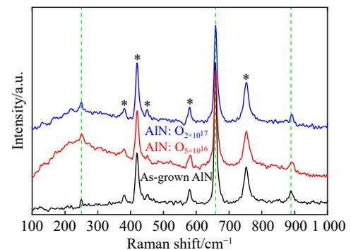
Fig. 2 Raman spectra for as-grown AlN, AlN:O<sub>5 $\times$ 10<sup>16</sup></sub>, and AlN:O<sub>2 $\times$ 10<sup>17</sup></sub>. The asterisks represent vibrational modes related to the sapphire substrate. The green dotted lines represent the first-order phonon modes of AlN  $E_2$  (low),  $E_2$  (high), and  $A_1$  (LO), respectively. (color online)
