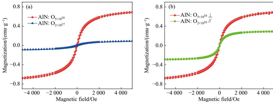
Fig. 5 (a) Room-temperature out-of-plane  $M$ - $H$  loops for AlN:O<sub>5×10<sup>16</sup></sub> and AlN:O<sub>2×10<sup>17</sup></sub>. The diamagnetic background signals were subtracted. The magnetization values were normalized by accounting for the masses of the AlN films. (b) Magnetic anisotropy of AlN:O<sub>5×10<sup>16</sup></sub>. (1 Oe=1000/(4 $\pi$ ) A/m)
