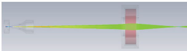
图3 CST 仿真束流轨迹图 Fig. 3 CST simulation beam trajectory diagram
